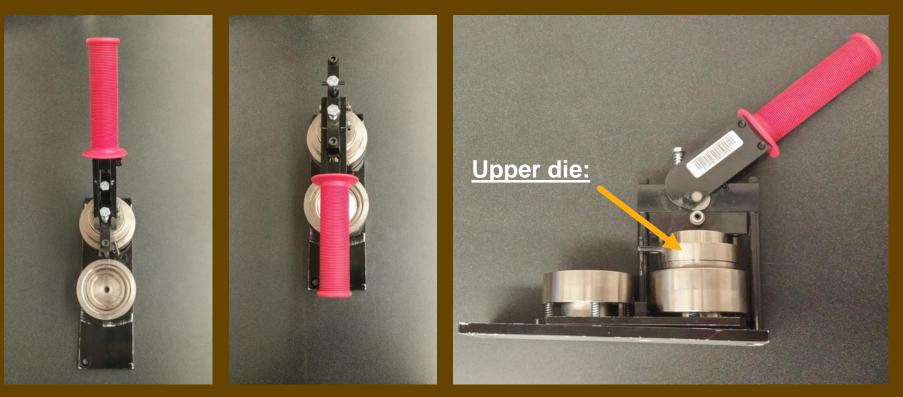
Place the loop holder sharp edge up inside the exposed crimp die.
