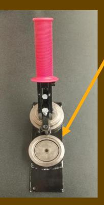
Pickup die: The flat surface ensures the shell, image and Mylar are level
